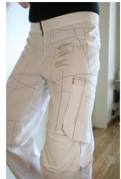
The Half-Proto may include a measurement chart which is printed on. For high-visibility and workwear garments, the Half-Proto can include the areas of fluorescent and reflective material by exposed surface. This option supports the approval process for class I – III certificates by the authorizing institutes. Logo's and graphic artwork in a line representation can be added.
